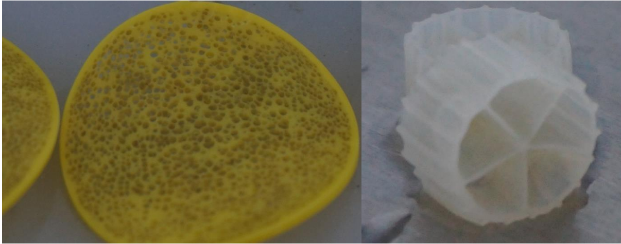
Figure 3: MBBR media types used in the study – Mutag BioChip 30(L) and K1 equivalent (R)
